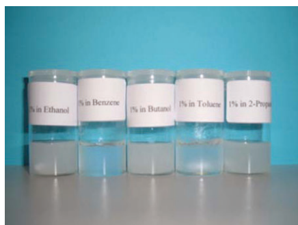
Fig. 2 Gels formed using the LMOG 1.
